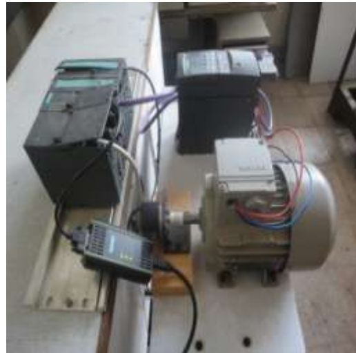
Fig.2 Connections between PLC, drive and motor.
